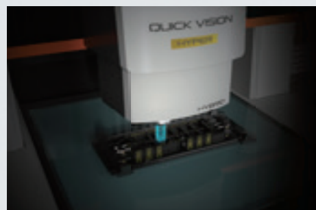
Example of measuring an engine control unit
